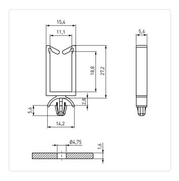
Bundle Diameter [mm]: 10,0-25,0 Color: Natural Height [mm]: 26.9 Material: PA 6.6 Material Group: **Plastic** Mounting Hole [mm]: 4.8 Panel Thickness [mm]: 1,6 mm Width [mm]: 15.9
