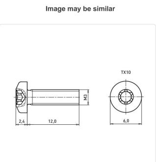
Actuator Size: Torx T10 DIN/ISO: ISO14583 Drive Type: **TORX**
