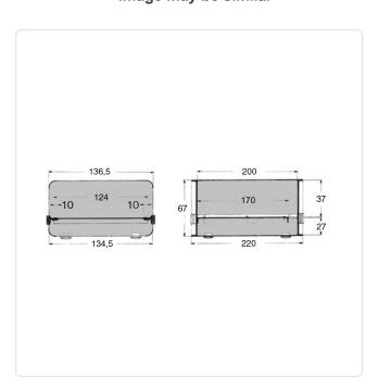
Color: Black Height [mm]: 67 Length [mm]: 220 Material: Steel Material Group: Steel Width [mm]: 136.5 Weight: 961g Conformities:
