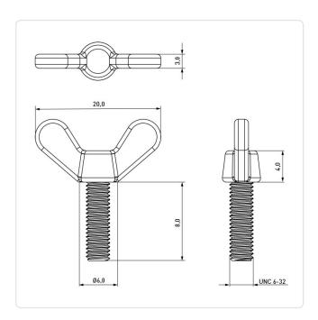
Color: Natural Flammability Class: UL94-V2 Head Diameter [mm]: 20 Length [mm]: PA 6.6
