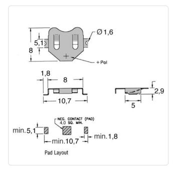
Battery Type: Cell Dia. 6mm
