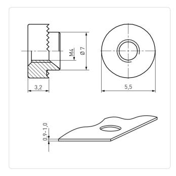
Finish: Plain Height [mm]: 3.2 Material: Steel Outer Diameter [mm]: 7 Panel Hole Ø [mm]: 5.5 Panel Thickness [mm]: 0,9 - 1,0 Thread Size: M4
