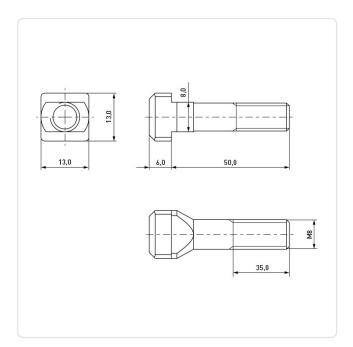
DIN/ISO: **DIN787** Plain Finish: Head Height [mm]:
