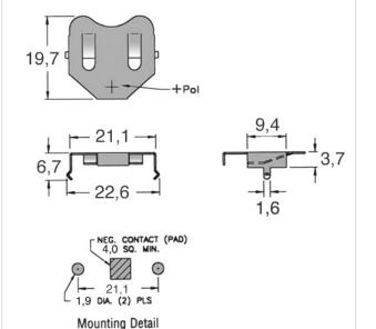
Battery Type: Cell Dia. 20mm Cell diameter [mm]: Ø 20.0 Finish: Nickel-Plated, 3 µm, E1E Height [mm]: 3.7 Material: **Phosphor Bronze Phosphor Bronze** Material Group: PCB Mounting Connection Model: No. Cells: 1 Weight: 0.97g Conformities: Reach RoHS SVHC
