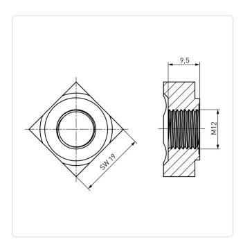
AF / OD [mm]: 19 DIN/ISO: **DIN928** Finish: Plain Height [mm]: 9.5 Steel Material: Thread Size: M12
