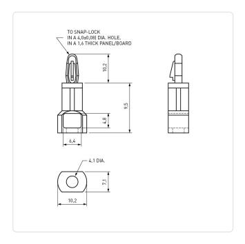
Color: Natural UL94-V2 Flammability Class: Length [mm]: 9.5 PA 6.6 Material: Material Group: **Plastic** PCB Hole Ø [mm]: PCB Thickness [mm]: 1,6 Panel Hole Ø [mm]: 4.1 Weight: 0.43g
