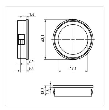
Color: Black Inner Diameter [mm]: 46 Material: PA 6.6 Material Group: Plastic Max. Panel Thickness [mm]: 6.4 Mounting Hole [mm]: 57.2 Weight: 9.9g Conformities:
