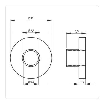
Color: Natural Flammability Class: UL94-V2 Height [mm]: 3.5 Inner Diameter [mm]: 8.2 Lug Diameter [mm]: 9.9 Material: PA 6.0 Material Group: Plastic
