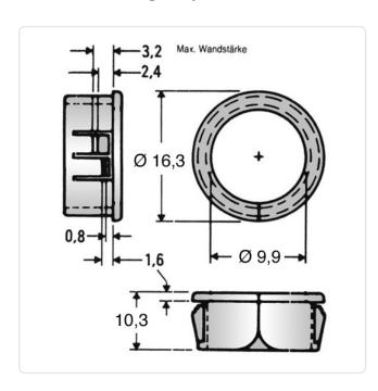
Color: Black Inner Diameter [mm]: 9.9 Material: PA 6.6 Plastic Material Group: Max. Panel Thickness [mm]: 3.2 Mounting Hole [mm]: 14.3 Outer Diameter [mm]: 16.3 Weight: 0.53g
