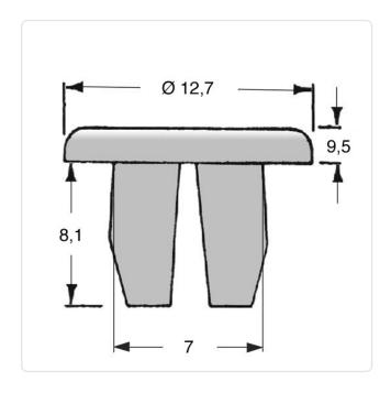
AF / OD [mm]: 12.7 Color: Natural Head Height [mm]: 9.5 Length [mm]: 8.1 Material: PA 6.6 Material Group: Plastic Panel Cutout [mm]: 7.0x7.4 Panel Thickness [mm]: 0,8-4,0 Thread Diameter [mm]: Ø 4.2 Weight: 1.5g Conformities:
