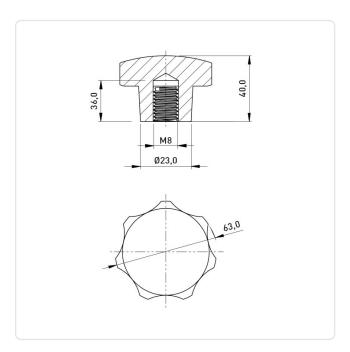
Color: Black Diameter [mm]: 63 Height [mm]: Material: PA 6.0 Material Group: Plastic Thread Size: M8 Weight: 35.7g
