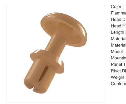
Color: Brown UL94-V2 Flammability Class: Head Diameter [mm]: 6.4 Head Height [mm]: 1.6 Length [mm]: 6.5 Material: PA 4.6 Material Group: Plastic Model: removable Mounting Hole Range [mm]: Ø 3.1-3.2 Panel Thickness [mm]: 4,0-5,0
