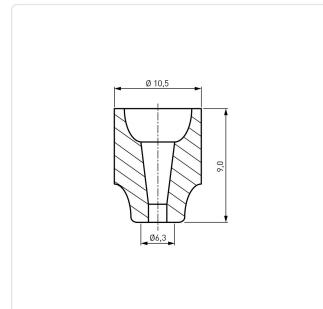
Inner Diameter [mm]: 6.3 Length [mm]: 9 Material: Ceramic C221 Material Group: Ceramic C221 Model: With Lug Outer Diameter [mm]: 10.5 Weight: 0.91g Conformities: Reach RoHS **SVHC**
