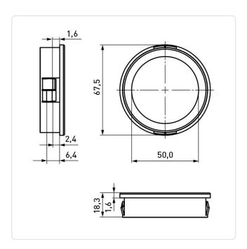
Color: Black Inner Diameter [mm]: 51 Material: PA 6.6 Material Group: Plastic Max. Panel Thickness [mm]: 6.4 Mounting Hole [mm]: 64 Weight: 13.38g
