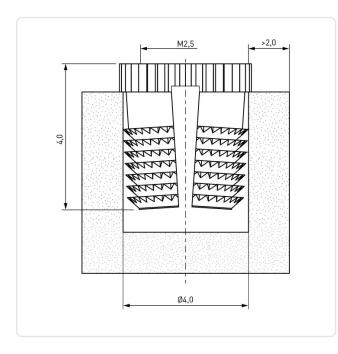
Finish: Plain Length [mm]: 4 Material: **Brass** Material Group: Brass Minimum Edge Distance [mm]: 2.0 Panel Hole Ø [mm]: Thread Size: M2.5
