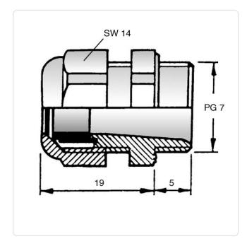
AF / OD [mm]: 14 Brass Material: Material Group: **Brass** Mounting Hole [mm]: 13 Panel Thickness Range [mm]: 3.0-6.5 Protection Code: **IP68** Thread Size: PG7 Weight: 9.96g
