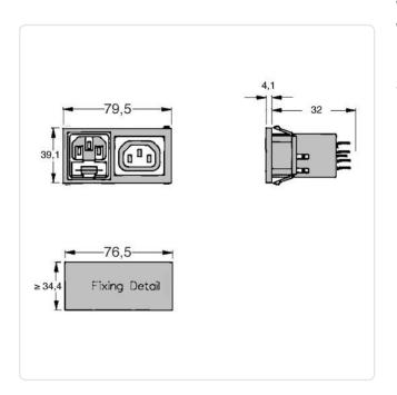
Amperage [A]: 10 Color: Black Connections: 6.3x0.8 Fuse Size [mm]: 5.0x20.0 Weight: 47g
