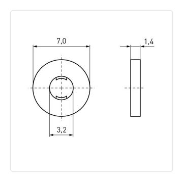
Color: Red For Thread Size: МЗ Height [mm]: 1.4 Inner Diameter [mm]: 3.2
