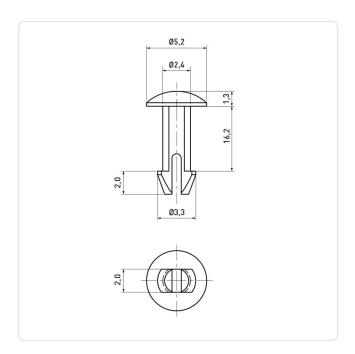
Color: Natural Flammability Class: UL94-V2 Head Diameter [mm]: 5.2 Material: PA 6.6 Material Group: **Plastic** Mounting Hole [mm]: 2.4 Weight: 0.11g
