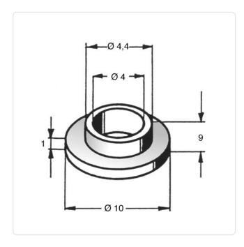
Color: Black Height [mm]: 9 Inner Diameter [mm]: 4 Lug Diameter [mm]: 4.4 Material: PA 6.6 Material Group: Plastic
