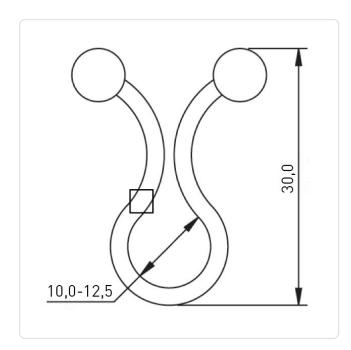
Bundle Diameter [mm]: 10,0-15,0 Color: Natural Flammability Class: UL94-V2 Material: PA 6.6 Material Group: **Plastic** Weight: 0.45g
