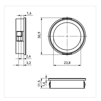
Color: Black Inner Diameter [mm]: 24 Material: PA 6.6 Material Group: Plastic Max. Panel Thickness [mm]: 3.2 Mounting Hole [mm]: 28 Weight: 2.62g
