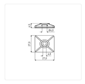
Cable Tie Width max. [mm]: 4.8 Color: Black Flammability Class: UL94-V2
