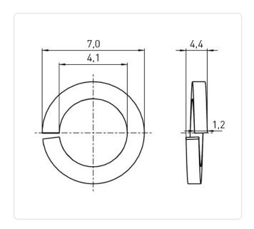
DIN/ISO: **DIN7980** Finish: Plain For Thread Size: M4 1.2 Height [mm]: Inner Diameter [mm]: 4.1
