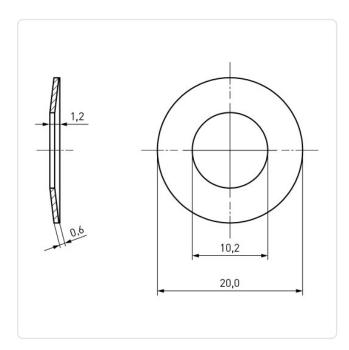
DIN/ISO: **DIN2093** Finish: Plain For Thread Size: M10 Height [mm]: 0.6 Inner Diameter [mm]: 10.2
