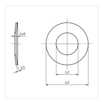
DIN/ISO: **DIN2093** Finish: Plain For Thread Size: M3 0.3 Height [mm]: Inner Diameter [mm]: 3.2
