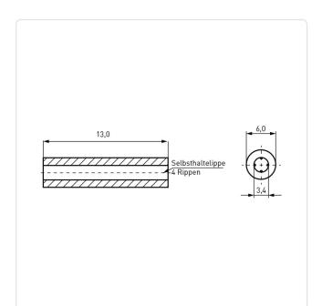
Color: Black Flammability Class: UL94-V2 For Thread Size: M3 Inner Diameter [mm]: 3.4 Length [mm]: 13 Material: PA 6.6 Material Group: Plastic
