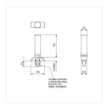
Color: Natural Flammability Class: UL94-V2 Length [mm]: 9.5 Material: PA 6.6 Material Group: **Plastic** Panel Hole Ø [mm]: 3.2 Panel Thickness [mm]: 0,8-2,0
