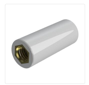
AF / OD [mm]: 12.7 Flammability Class: UL94-HB Length [mm]: 35 PA 6.6 Material: Material Group: **Plastic** Profile: Round Thread 1 Length [mm]: 12.7 Thread 1 Size: M6 Thread 2 Length [mm]: 12.7
