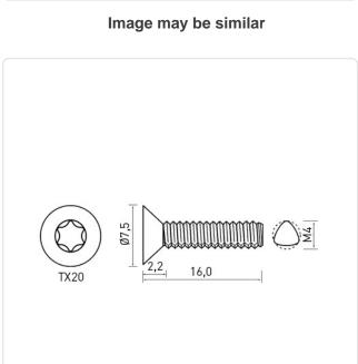
Actuator Size: Torx T20 DIN/ISO: DIN7500-M Drive Type: **TORX**
