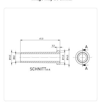
Color: Black Inner Diameter [mm]: 7.9 Material: **PVC** Material Group: Plastic Mounting Hole [mm]: 11 Panel Thickness [mm]: 0 Weight: 2.84g
