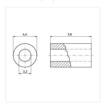
Color: White Flammability Class: UL94-V2 For Thread Size: М3 Inner Diameter [mm]: 3.2 Length [mm]: 3.8 Material: PA 6.0 Material Group: Plastic Outer Diameter [mm]: 6.4 Weight: 0.11g
