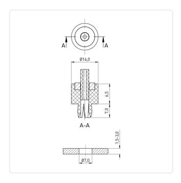
Color: Black Diameter [mm]: 16 Height [mm]: 6.5 Material: PA 6.0 Panel Hole Ø [mm]: Panel Thickness [mm]: 1,5-3,0 Weight: 1.39g
