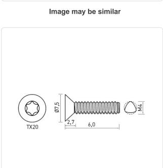
Actuator Size: Torx T20 DIN/ISO: DIN7500-M Drive Type: **TORX** Plain Finish:
