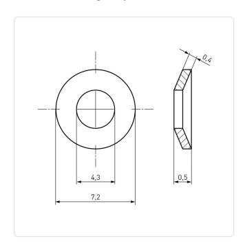
Finish: Plain For Thread Size: M4 0.4 Height [mm]: Inner Diameter [mm]: 4.3
