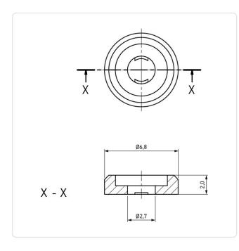
Color: Black For Thread Size: M2.5 Height [mm]: Inner Diameter [mm]: 2.7 Material: PA 6 Material Group: Plastic Outer Diameter [mm]: 6.8 Weight: 0.05g
