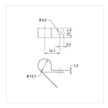
Bundle Diameter [mm]: 12,7 Color: Natural Distance Middle/Middle [mm]: 14.1 Flammability Class: UL94-V2 Material: PA 6.6 Mounting Hole [mm]: 5.2 Thickness [mm]: 1.3 Width [mm]: 12.7 Weight: 1.17g
