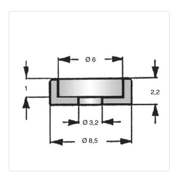
Color: White For Thread Size: МЗ Height [mm]: 2.2 Inner Diameter [mm]: 3.2 Material: PA 6 Material Group: Plastic Outer Diameter [mm]: 8.5 Weight: 0.09g
