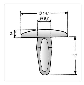
Color: Black Flammability Class: UL94-V2 Head Diameter [mm]: 14.1 PA 6.6 Material: Material Group: **Plastic**
