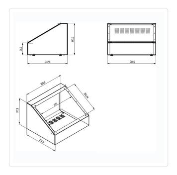
Color: Blue Height [mm]: 197 Length [mm]: 247 Material: Steel Material Group: Steel
