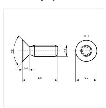
Actuator Size: Torx T10 DIN/ISO: ISO14581 Drive Type: **TORX**
