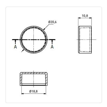
Color: Gray Head Height [mm]: 10.8 Inner Diameter [mm]: 18.8 Material: PA 6.0 Material Group: **Plastic**
