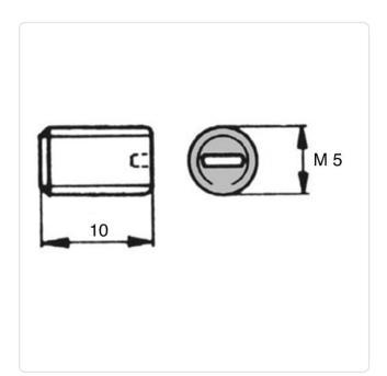
Color: Natural DIN/ISO: ISO4766 Drive Type: Slotted Flammability Class: UL94-V2 Length [mm]: 10 Material: PA 6.6 Material Group: Plastic Point Type: Flat Point Thread Size: M5
