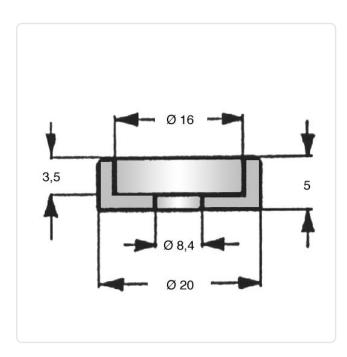
Color: White For Thread Size: M8 Height [mm]: Inner Diameter [mm]: 8.4 Material: PA 6 Material Group: Plastic Outer Diameter [mm]: 20 Weight: 0.85g
