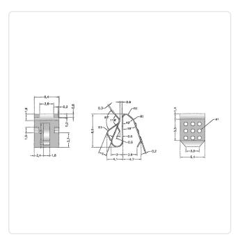
Battery Type:AAA-MicroFinish:Nickel-Plated, 3 µm, E1EMaterial:Spring SteelMaterial Group:SteelWidth [mm]:6.4Weight:0.42gConformities:ReachReachRoHSConformities:Reach
