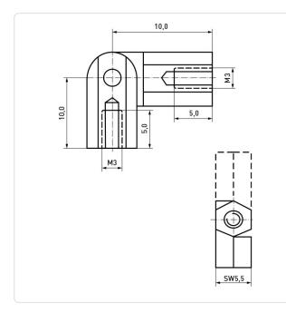
Finish: Galvanized, Blue, 5 µm, A2K Leg Length 1 [mm]: 10 Leg Length 2 [mm]: 10 Length [mm]: 20 Material: Steel Material Group: Steel Model: Female/Female M3 Thread 1 Size: Thread 2 Size: М3 Weight: 3.02g Conformities: Reach RoHS
